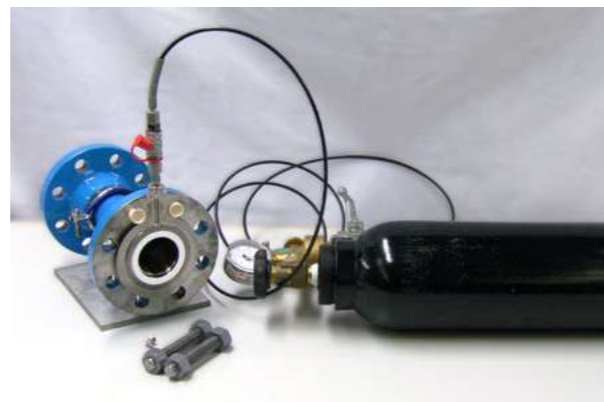
Typical set up of Alba-RIG™ leak test using nitrogen bottle
